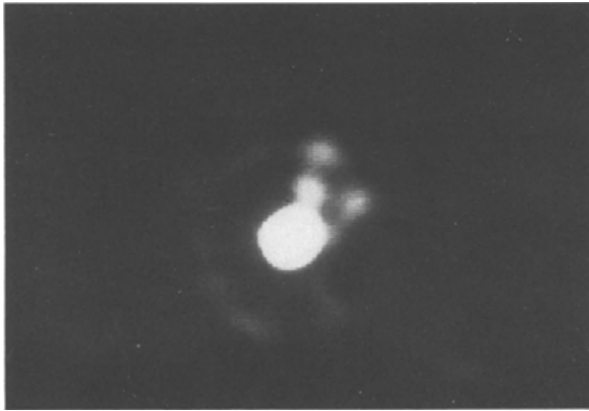
Fig. 4. Speckle masking observation of Eta Carinae at \lambda \sim 850 \text{ nm} . The diffraction-limited image was reconstructed from 300 speckle interferograms recorded with the 2.2-m ESO/MPG telescope. The separations of the three faint star-like objects are 0.11'' , 0.18'' , and 0.21'' .
