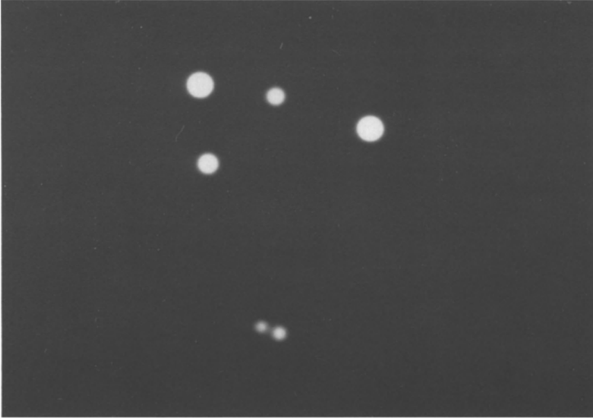
Fig. 3. Speckle masking observation of the central object in the giant H II region NGC 3603. The diffraction-limited image was reconstructed from 300 speckle interferograms recorded with the 2.2-m ESO/MPG telescope. The separation of the close double star at the bottom is about 0.08'' .
